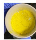
Fig9: Reaction deprotonated ylide and 9-Anthraldehyde. Vacuum filtered with water to remove inorganic salts. Organic solid remains.
