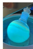
Fig7: Round bottom flask filled with fractions from flash column under UV lamp during solvent evaporation.
