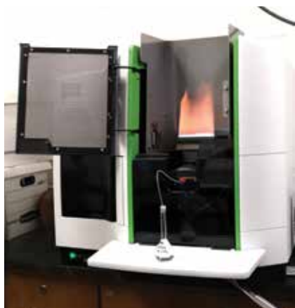
▲ The Atomic Absorption Spectrophotometer used in Obando's project
